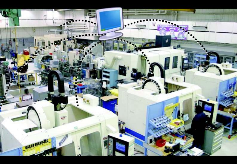
NCnet DNC system transfers programs between a PC and multiple CNC machines through a wired or wireless network.
